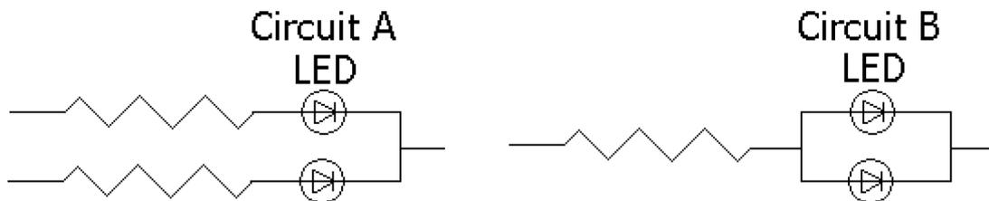
(a) Circuit A: it is recommended circuit.
