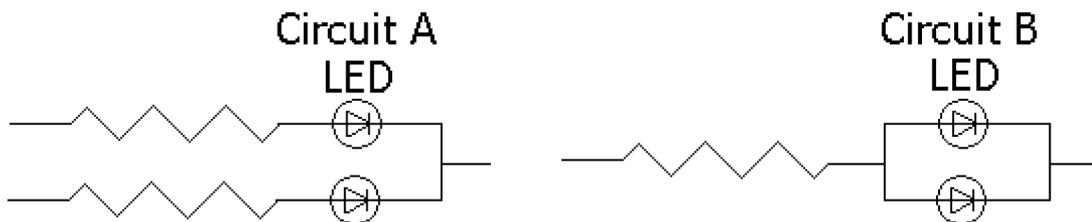
(a) Circuit A: it is recommended circuit.
