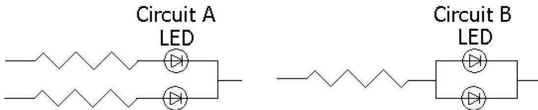
(a) Circuit A: it is recommended circuit.
